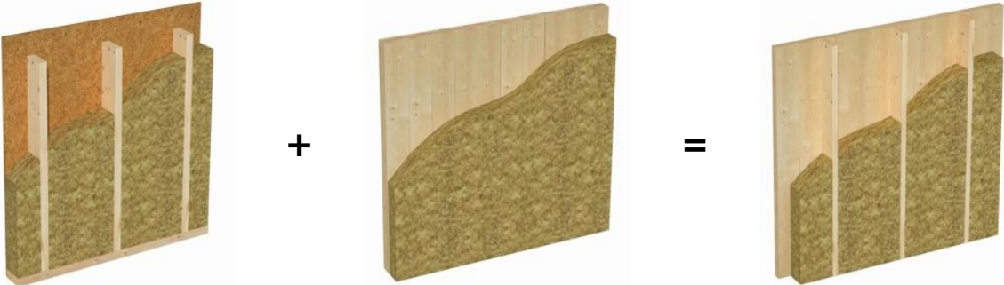
Figure 3: Combining a light timber frame with a CLT panel results in an effective XR-lam wall element
