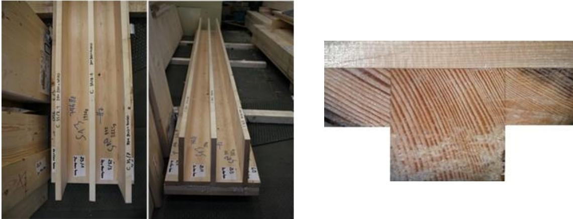
Figure 8: One of the final specimens and the glue lines around the rib
